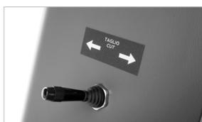
Pneumatic cross cut of material after rewinding
