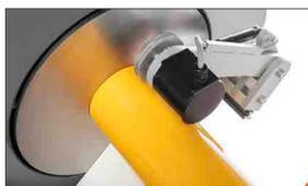
Encoder for measuring the rewind meters
