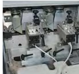
Milling unit before bending rollers
