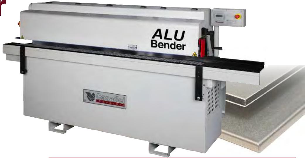
Automatic chain feeding milling and bending machine
