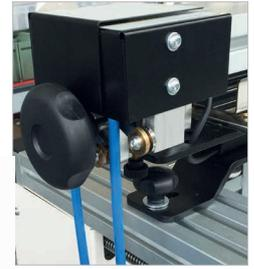
Supports profile with hollow chamber for the water-cooling
