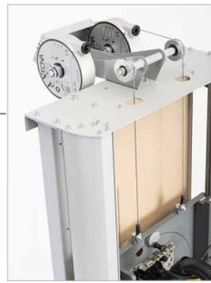
Mechanical balancing system to facilitate the movement of the cutting unit (in the picture is represented the horizontal balancing -optional- useful to reduce the height of the machine)
