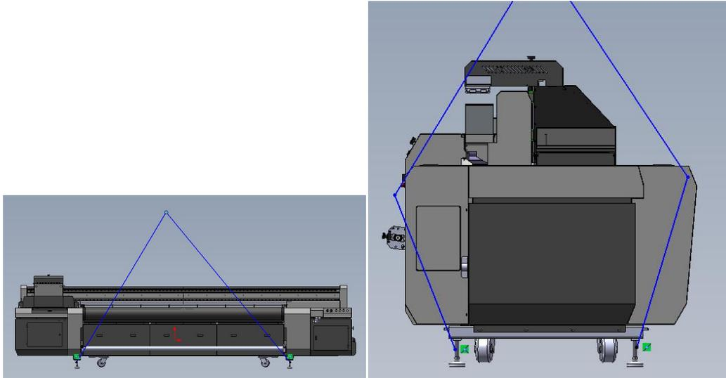
If lifting to upper floors needed, please mount the hoisting rope to the foot cups according to image 1 and 2, then proceed hoisting operation.
