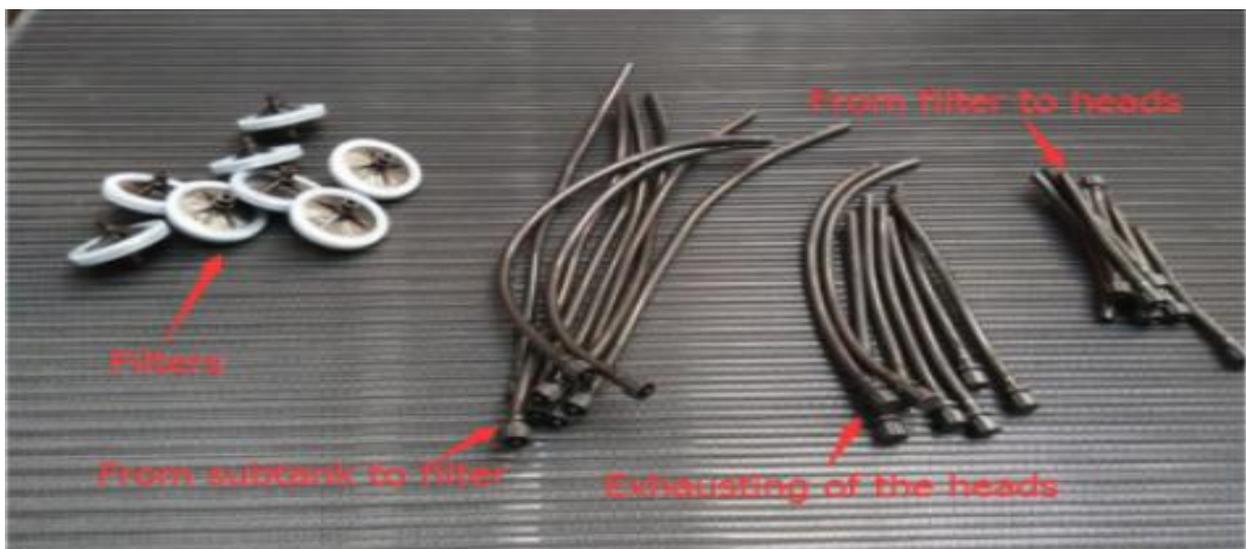
2 Assembling head inlet and outlet ink tube.
