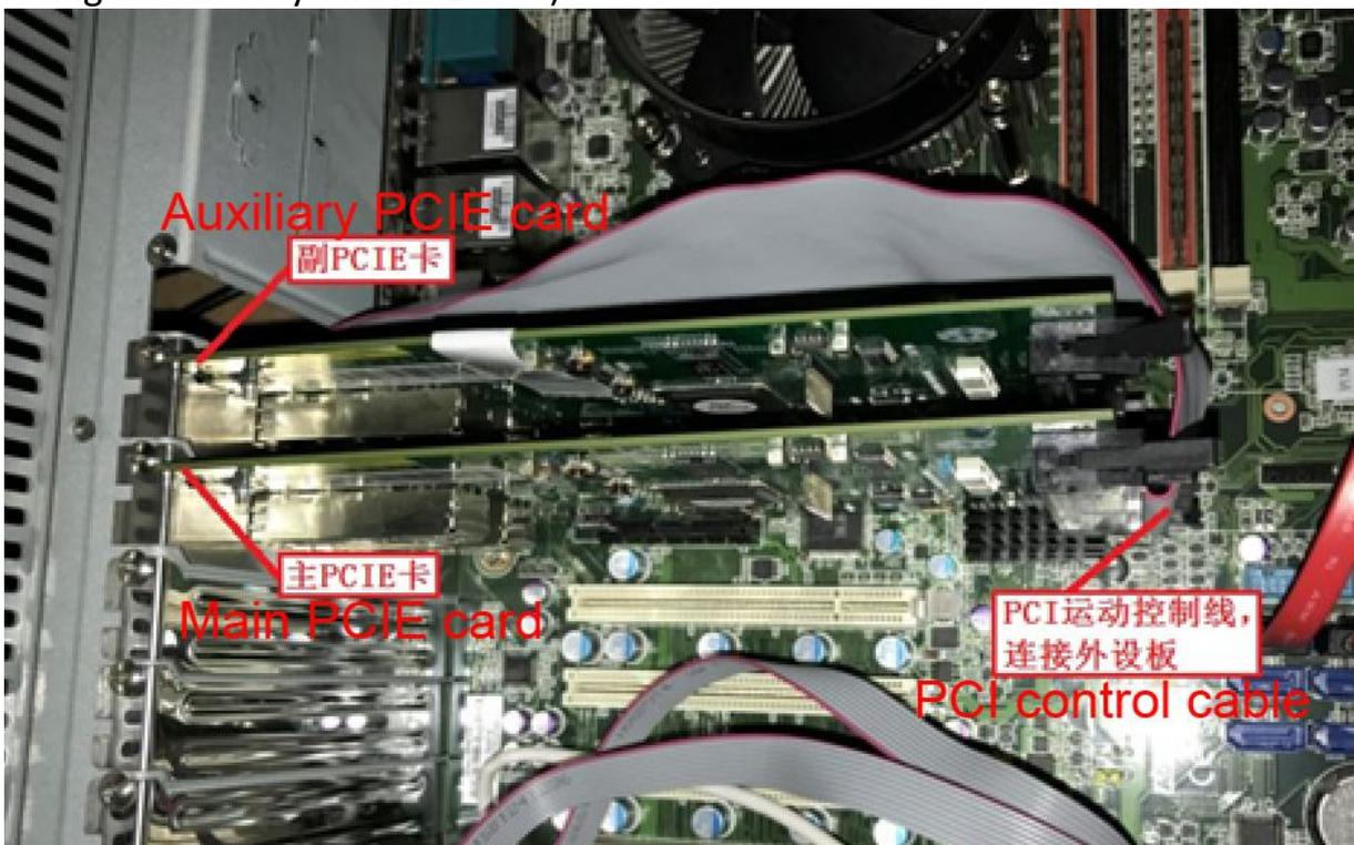
Install the PCIE card to the PC. Connect the movement control cable with the PCIE card and external device control board. Use the PC to connect the fiber cable for data transfer.
