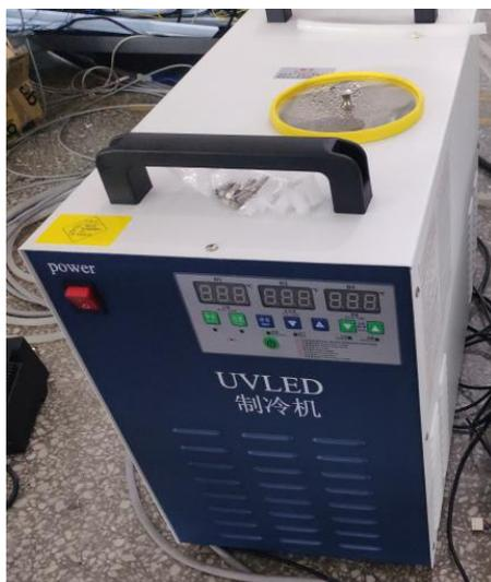
Connect the cooling circulation tube to the water hose. Then open the water-IN valve. Connect the power unit to 220V power and start the chiller working. Finally add the pure water(temp above 10°C) or anti-freezing water (temp under 10°C)
