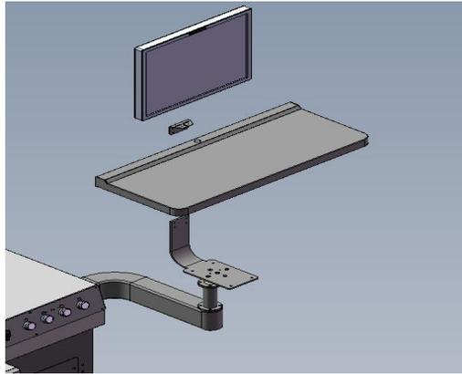
Install the display and PC according to the above picture and put the USB cable, PC start cable, display signal cable and power cable into the crate.
