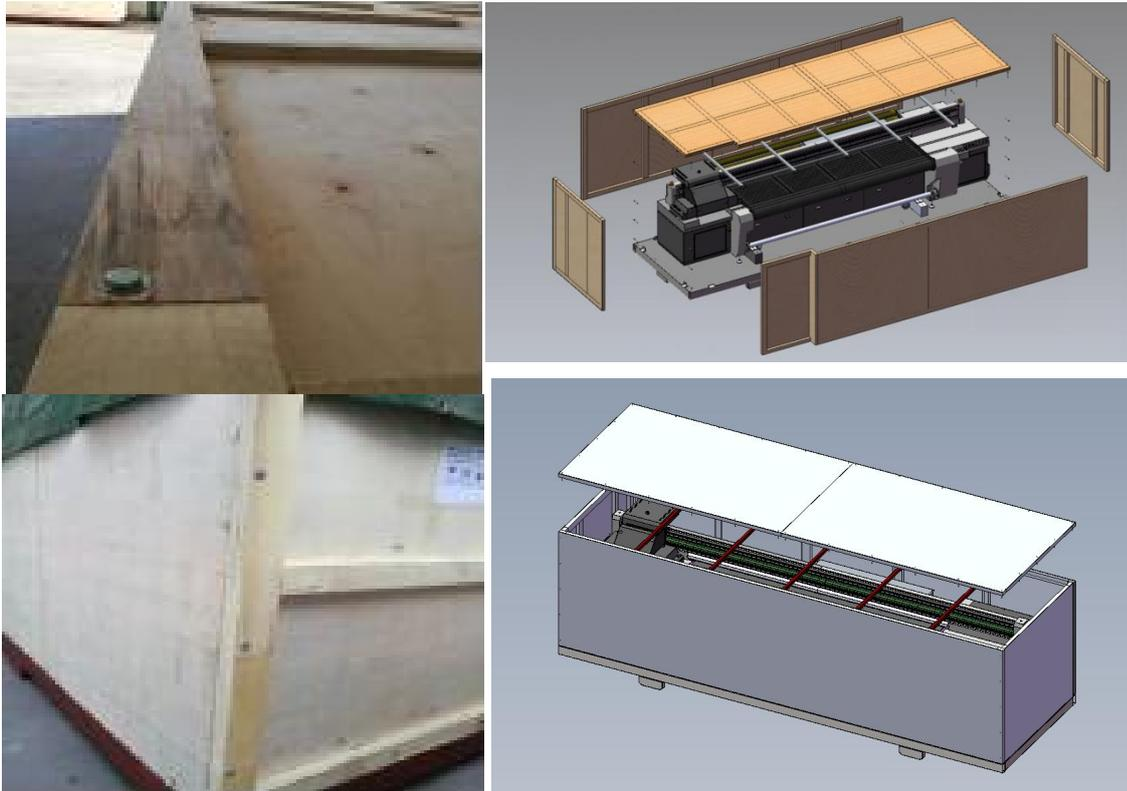
1. First remove the screws on the top of box and the upper plate. then remove five red mounted bars. In order to avoid the damage from the bar against the machine, do remember hold the bar before unscrew the screws.
