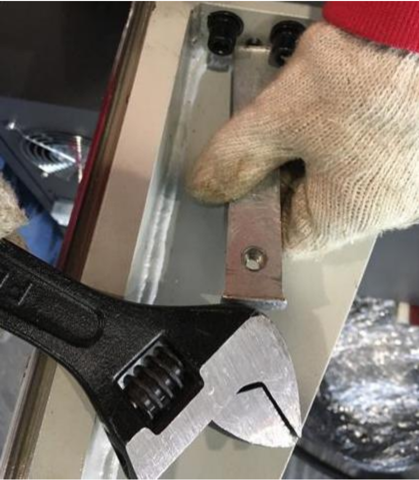
D. Mount the guide rail screw.
