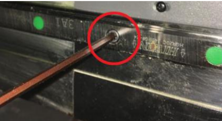
D. Mount the guide rail screw.
