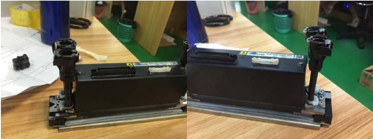
4 Finish the connecting between sub tank to heads and fix the printhead
