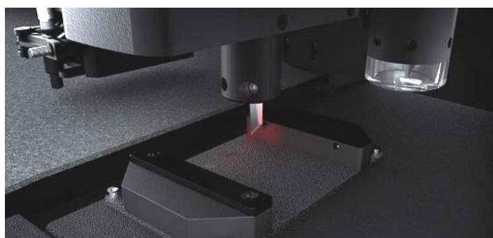
When starting up the table or after a tool change, the down position of each installed knife is measured to detect changes and avoid operator errors if the ADC is installed.
