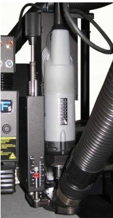
The router module has a motor capable of handling most used solid boards in the graphic and sign industry.
