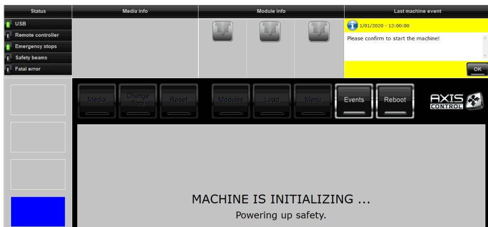
Click **OK** to proceed with the startup sequence. In the next step the emergency buttons will be checked and after that the safety trip switches and the safety light beams.
